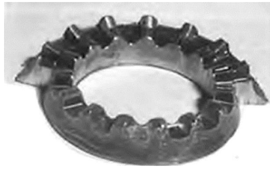
Fig. 7. View of the rings after direct extrusion of the end profile by the extrusion method and cutting off a part of the external ring.
