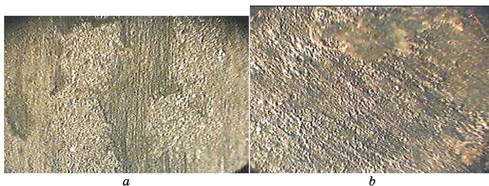
Fig. 5. The friction surface: on the glass at SN pole ( a ), on steel 45 in the direction of SN magnetic field ( b ), \times 100 .
